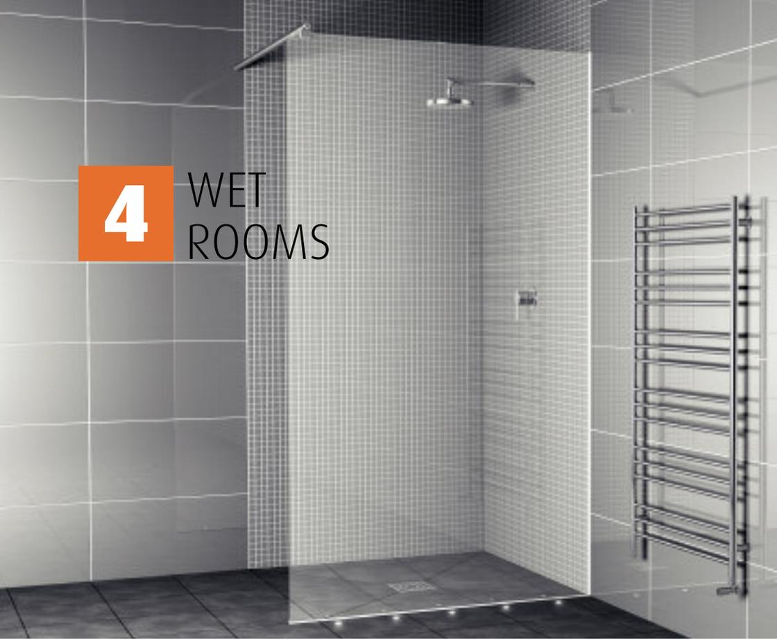
For wet rooms, always lay NO MORE PLY boards on the floor before overboarding the walls. Waterproof all joints with Mega Strength Polyurethane Adhesive. To make NO MORE PLY boards completely waterproof, coat the completed NO MORE PLY surface with two coats of SBR primer (one part SBR to three parts water).
