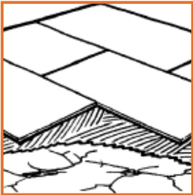
a) NO MORE PLY is ideal for covering dirty, cracked, worn out concrete floors. Always remove loose material, clean thoroughly and prime with one coat of SBR primer (one part SBR to three parts water) before laying NO MORE PLY.
